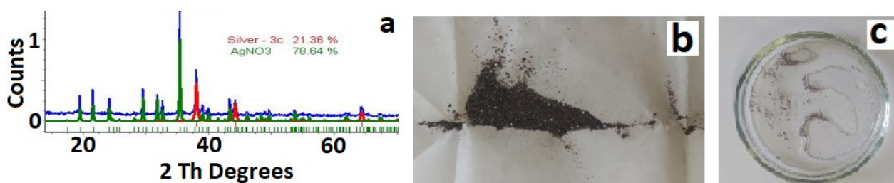
Fig. 1 (a) XRD pattern of composite Fhy-Ag 2 ; (b) Fhy-Ag composite nanopowder; (c) Fhy-Ag composite nanoparticles on the surface of H 2 O.
