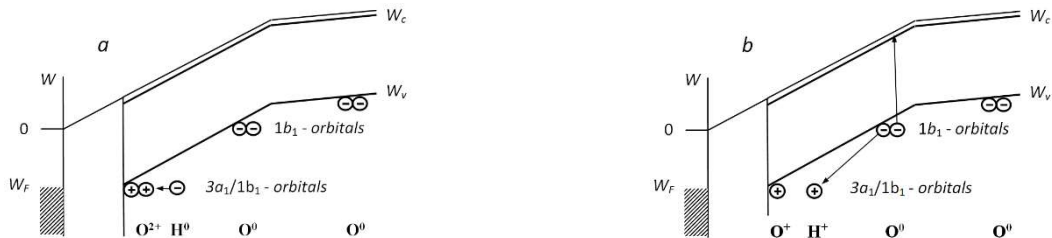
Fig. 2. Resonance (a) and Auger (b) transitions in water in strong electric field. W_F – Fermi level of metal, W_c – conduction band bottom energy level, W_v – valence band top energy level.
