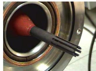
Fig. 14. Photo of the 8-emitter graphite cathode
