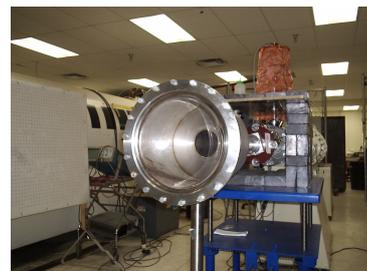
Fig. 15. Photo of the output antenna and vacuum window of the SINUS-6 accelerator
