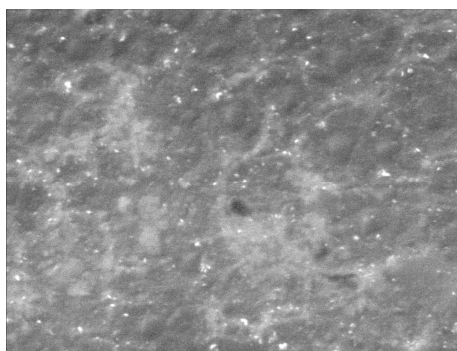
Fig. 1. The SEM image of Ca-P coating prepared by rf-magnetron sputtering on the titanium substrate. Time of deposition is 80 min. Magnification is 10000
