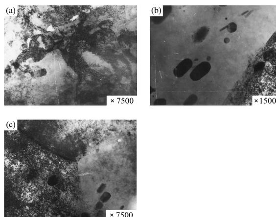
Fig. 2. Microstructure of initial (a, b) and annealed (c) AMg6 alloy
