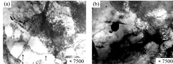
Fig. 4. Image of subgrain structure of AMg6 alloy irradiated with  $\text{Ar}^+$  ions:  $E=40 \text{keV}$ ,  $j=200 \mu\text{A}/\text{cm}^2$ ,  $D=1.7 \cdot 10^{17} \text{cm}^{-2}$
