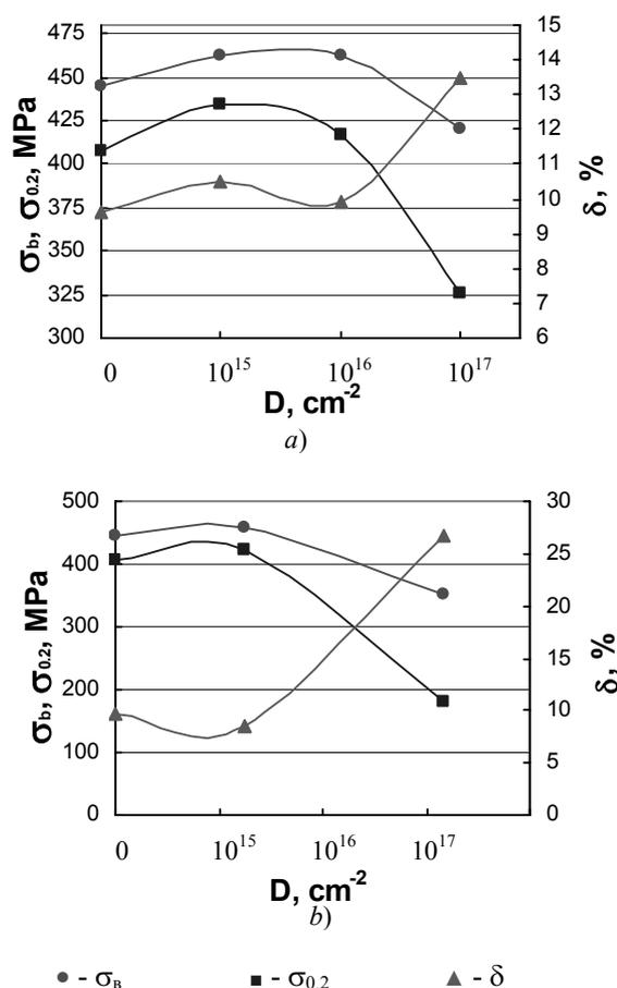
Fig. 1. Relationship between dose, ultimate stress  $\sigma_s$ , yield strength  $\sigma_{0.2}$  and unit elongation for AMg6 alloy under irradiation with Ar<sup>+</sup> ions: a –  $E=20 \text{ keV}$ ,  $j=150 \mu\text{A}/\text{cm}^2$ ; b –  $E=40 \text{ keV}$ ,  $j=200 \mu\text{A}/\text{cm}^2$
