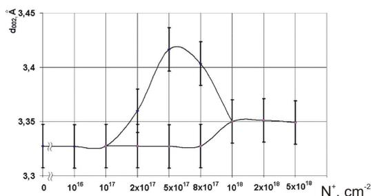
Fig. 3. Dependence of interplane distance  $d_{002}$  from a dose of ion irradiation
