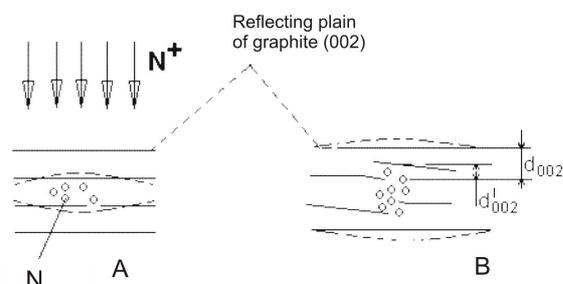
Fig. 4. Model of structure near surface layer of graphite after ion irradiation. A – the initial moment of an ion irradiation (dose  $N^+ < 10^{16} \text{ cm}^{-2}$ ); B – structure of near surface layer after dose  $N^+ \approx 2 \cdot 10^{17} \div 10^{18} \text{ cm}^{-2}$
