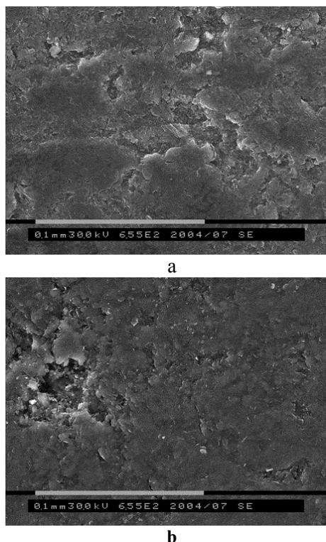
Fig. 6. Topography of graphite surface after an nitrogen ion irradiation. a –  $10^{16} \text{ cm}^{-2}$ , with small craters; b –  $2 \cdot 10^{17} \text{ cm}^{-2}$ , with large crater
