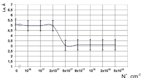
Fig. 5. Dependence of sizes of crystalline particle  $L_a$  as a function of  $N^+$ -ions dose
