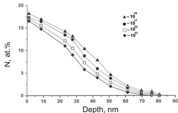
Fig. 1. Change of concentration of nitrogen in graphite after ion irradiation
