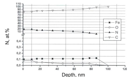
Fig. 2. Change of concentration impurities in a near-surface layer of graphite after an ion irradiation
