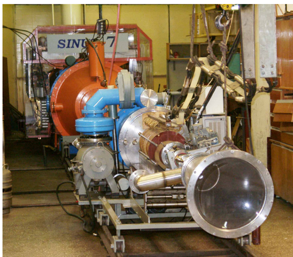
Fig. 2. The SINUS-7 electron accelerator in high-power BWO experiments
