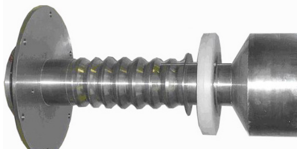
Fig. 3. Electrodynamic system of an S-band relativistic BWO with resonant reflector
