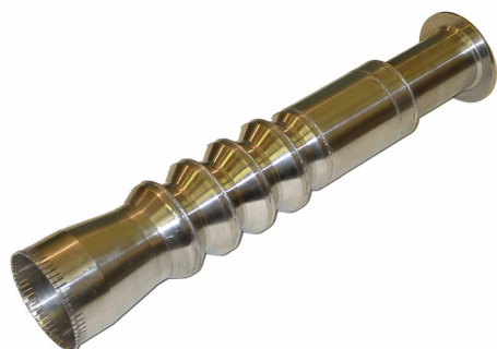
Fig. 2. Electrodynamic system of the resonant BWO
