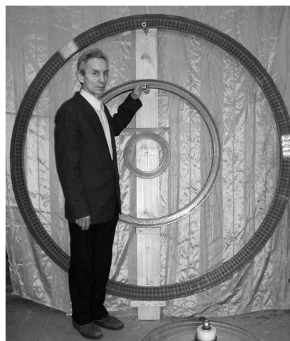
Fig. 2. Magnetic cores produced at HCEI. The largest in the photograph is one of 4 core rings for LTDZ
