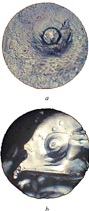
Fig. 4. Micrographs of Zr (a) and Cr (b) specimen surface treated by IPEB ( w = 32 \text{ J}\cdot\text{cm}^{-2} , n = 1 pulse) \times 400
